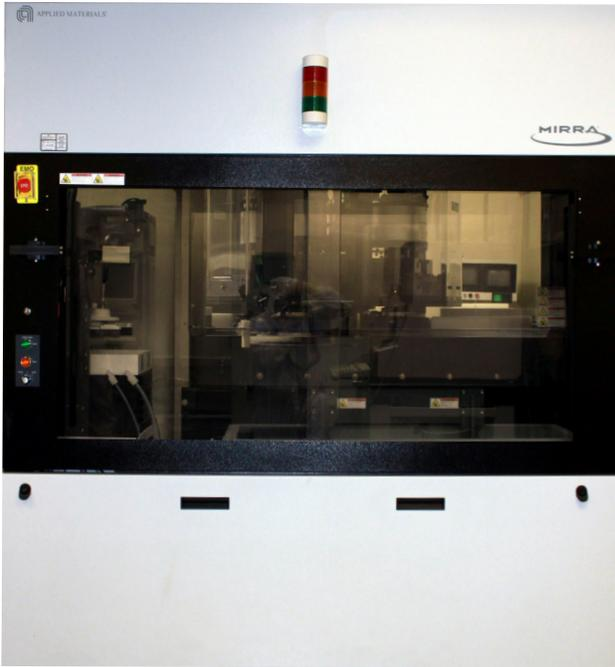
The Applied Materials Mirra CMP Tool is a Dry In - Wet Out (DI-WO) type of CMP machine which incorporates three polishing platens. The four wafer carriers are supported by a carousel transfer mechanism that moves the wafers through a one, two, or three step polishing process. It will process wafers from 150 to 200mm in diameter, and can be used for the planarization of thin films such as oxide, tungsten, and Polysilicon.
