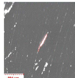
Scratches from Si wafer backside thinning
