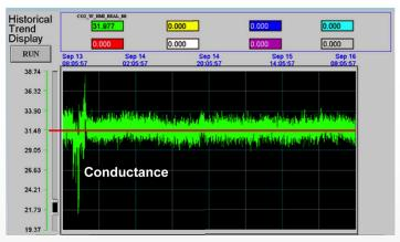
The Trusval CO<sub>2</sub>-DIW system delivers exceptionally consistent and stable CO2-saturated DI water at high volume. After initial setup and adjustment, the graph shows the delivery of process C0<sub>2</sub>-DI water at 31.5 microsiemens of measured conductance with a range of 2 microsiemens at a flow rate of 50 liters per minute.
