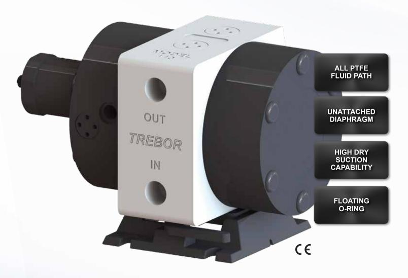
Years of proven reliability make Trebor's Model 110 pump an industry standard for lower flow, high-purity chemical pumping applications. The Model 110 is an air-operated, double-diaphragm pump that uses only virgin PTFE and PFA materials in the fluid path, making it compatible with virtually all process chemicals. The center fluid cavity and internal air control valves make this one of the smallest pumps on the market for its capacity.
